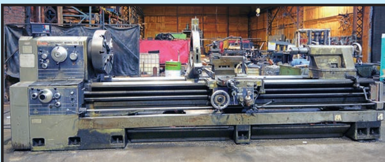
MAZAK 34" X 132" GAP BED ENGINE LATHE
