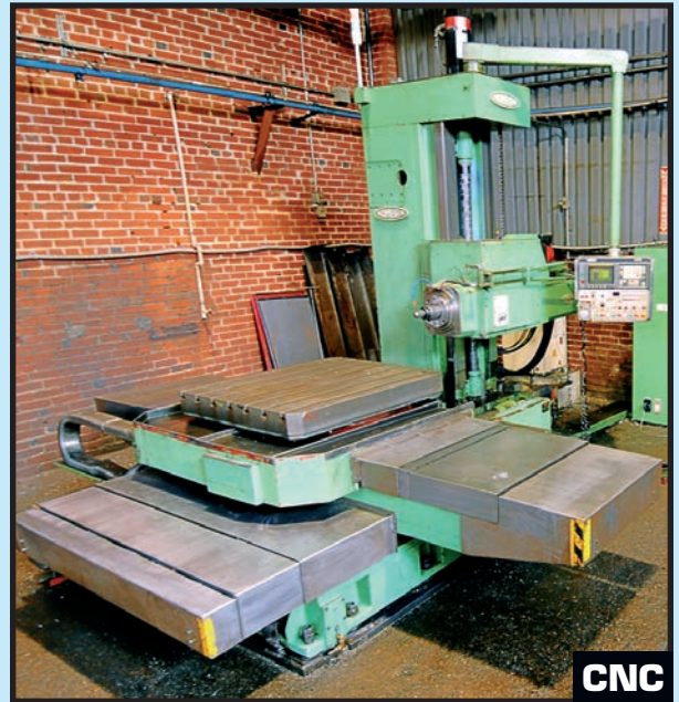
NOMURA 4" CNC HORIZONTAL BORING MILL
