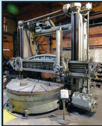
SELLERS 120" DOUBLE-COLUMN VERTICAL BORING MILL
