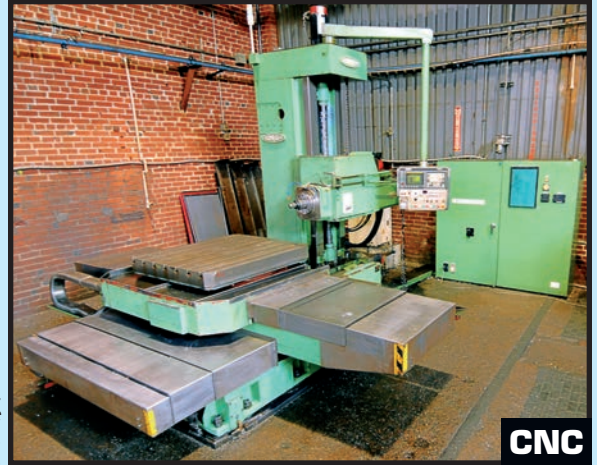
> NOMURA 4" CNC HORIZONTAL BORING MILL
