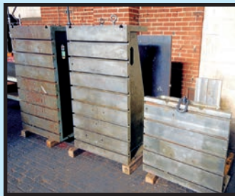
PARTIAL VIEW OF ANGLE PLATES
