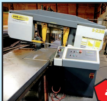
HYD-MECH MDL. S23A AUTOMATIC HORIZONTAL BANDSAW
