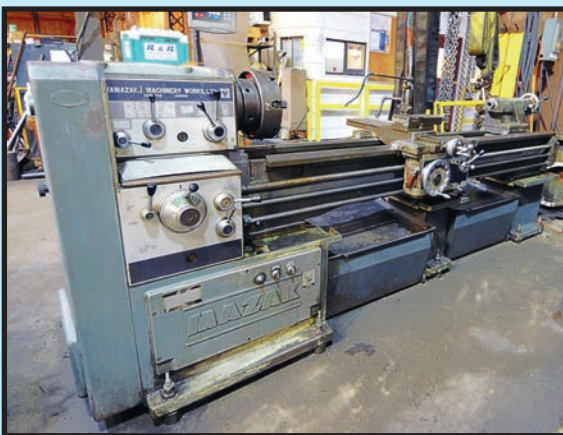
MAZAK 18" X 80" GAP BED ENGINE LATHE
