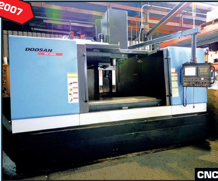
DOOSAN MDL. MV6030 CNC VERTICAL MACHINING CENTER
