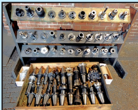
PARTIAL VIEW OF CAT-50 SPINDLE TOOLING
