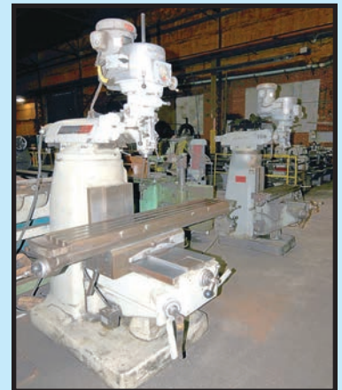
PARTIAL VIEW OF VERTICAL TURRET MILLS
