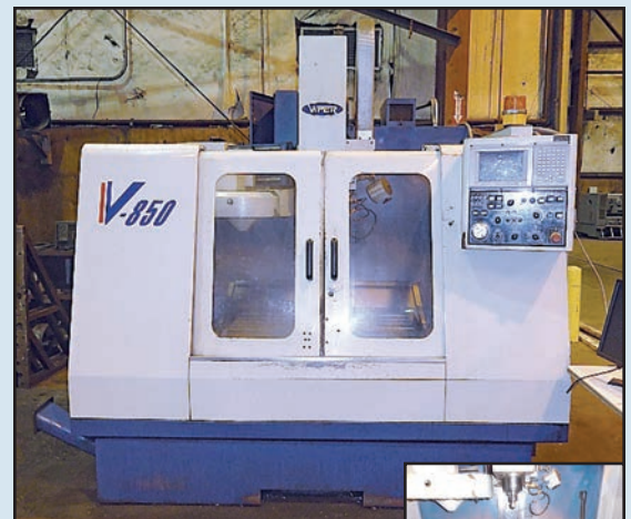
VIPER VMC , Mdl. 850-P, X=32", Y=20", Z=24.8", 32" x 18" table, Cat 40 tooling, 20-ATC, 10 HP, 8,000 RPM, w/Meldas M500 Series control, SN 912804-004, 1997.
