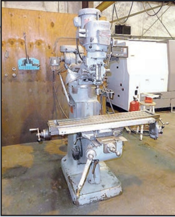
BRIDGEPORT Series I Mill , 9" x 48" table, VS, 2-axis DRO, PF@X, 2 HP, SN 231671.
