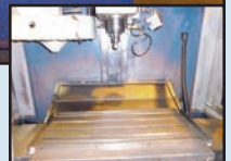
VIPER VMC , Mdl. 850-P, X=32", Y=20", Z=24.8", 32" x 18" table, Cat 40 tooling, 20-ATC, 10 HP, 8,000 RPM, w/Meldas M500 Series control, SN 912804-004, 1997.
