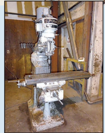
SUPERMAX Vertical Mill , 9" x 43" table, SN 81-047140.
