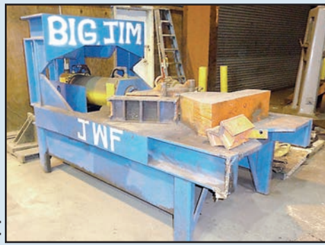
Bulldozer Press (BIG JIM press), 150-ton cap. (set up for tube bending).
