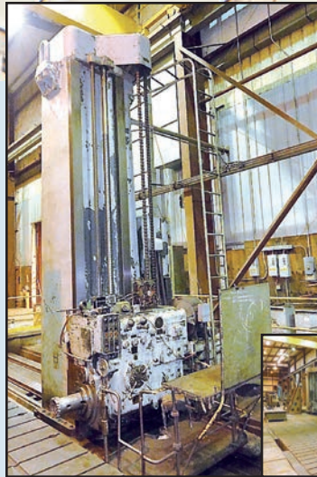
GIDDINGS & LEWIS 570 F Horizontal Boring Mill , 7" spindle, #7 Morse taper, X=288", Y=192", Z=144" vertical, 31" runway, w/Trak i02 2-axis DRO, SN 8658.
