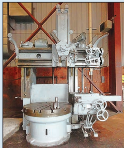
KING Vertical Turret Lathe , swivel turret head, side head, 42" face plate w/boring mill jaws, 58" swing, 25 HP, work height U/R 43", 3-98 RPM, SN N/A.
