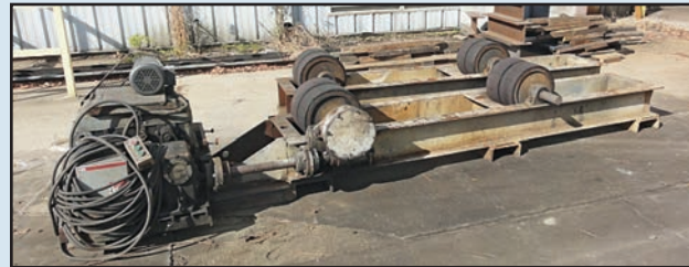
RANSOME Power Turning Rolls , 50-ton cap., SN 8678.
