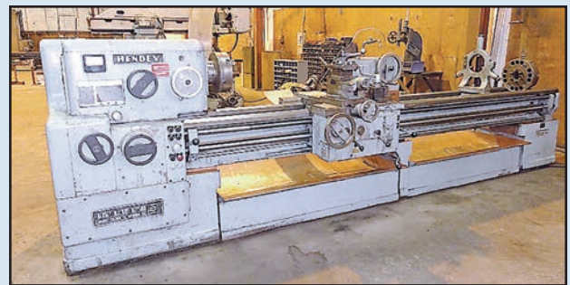
HENDEY Lathe , Mdl. 2516x126, 25" swing, 120" DBC, 2" spindle bore, 13-1,500 RPM, 20 HP, TS, SR, 12" 3-jaw chuck, SN DHL20.
