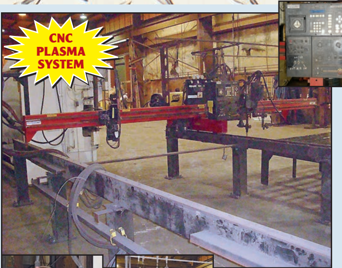
MG CNC "Apollo" Plasma System , 10' x 20' table, SN AP8x8PC/NC-96-3164, System 80 CNC controls, (1) oxy head, (1) plasma head, (1) tracing head w/Easb Powercut 1500 power source, 1-1/2".
