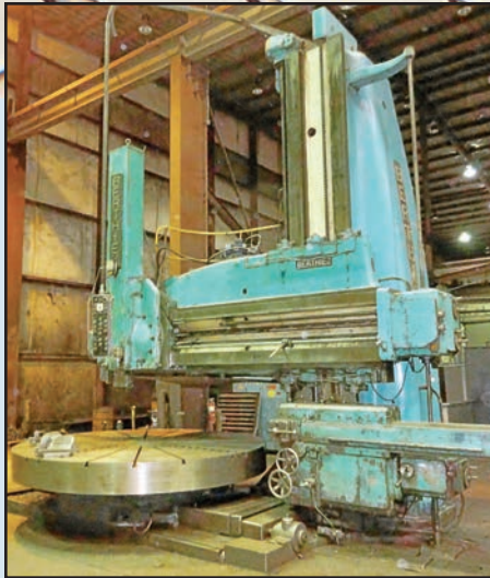
BERTHIEZ Vertical Boring Lathe , Mdl. 9135, 130" face plate, 196.85" swing, work height U/R 135", w/side head and RAM, boring mill jaws, pendant control and sliding table, SN 09030.
