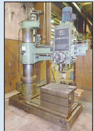
< AMERICAN Hole Wizard Radial Drill , 17" column x 6" arm, 44" x 60" box table, 30" x 20" table, #5 Morse taper, 1,200 max. RPM.
