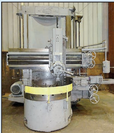
BULLARD Cutmaster Vertical Turret Lathe , swivel turret head, side head, 54" chuck, 62" swing, 30 HP, work height U/R 70", 4.5-160 RPM, pendant control, SN 25848.
